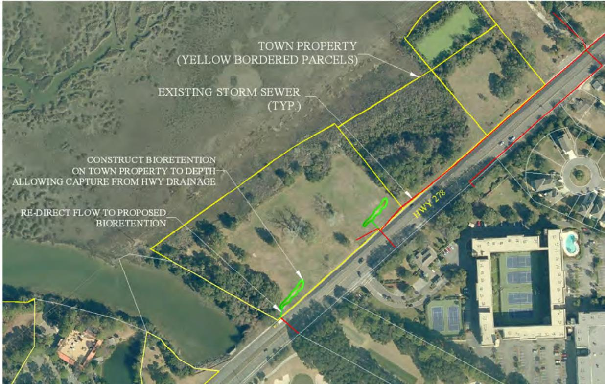
**Figure 8 – Bioretention BMP to treat small areas of the existing highway**
