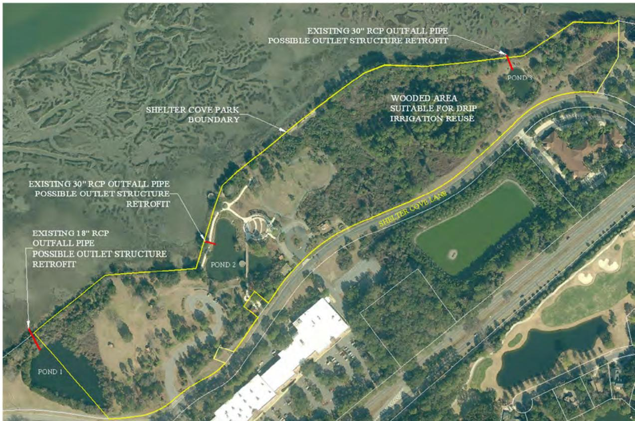
Figure 4 – Shelter Cove Park: Possible retrofits include pond outlet structures, pond littoral shelves, irrigation reuse in landscaped areas, and rainwater drip field disposal in wooded areas.
