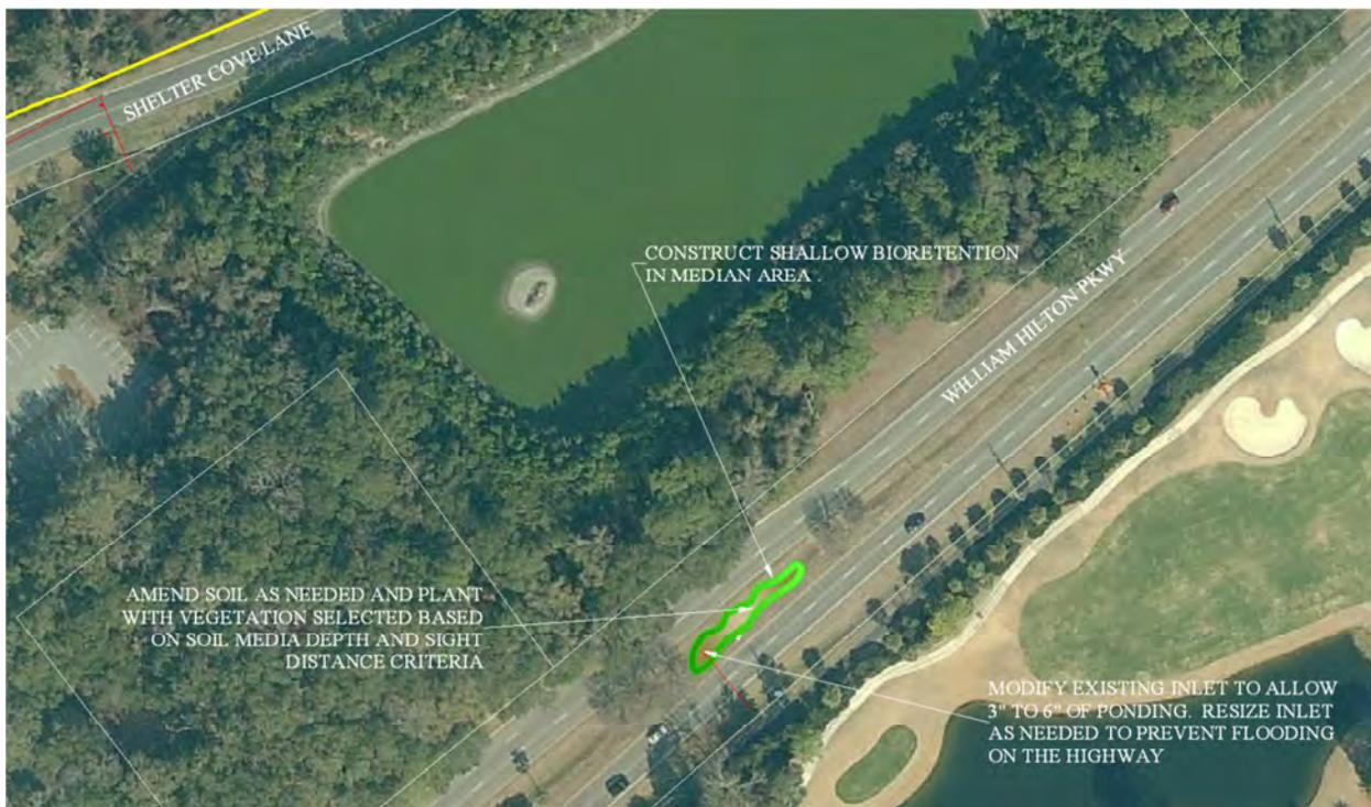
**Figure 11 – Bioretention BMP option within William Hilton Pkwy median**
